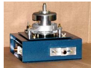
Permanent Magnet Turbine
